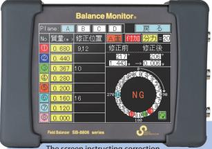
The screen instructing correction using the specified weight
